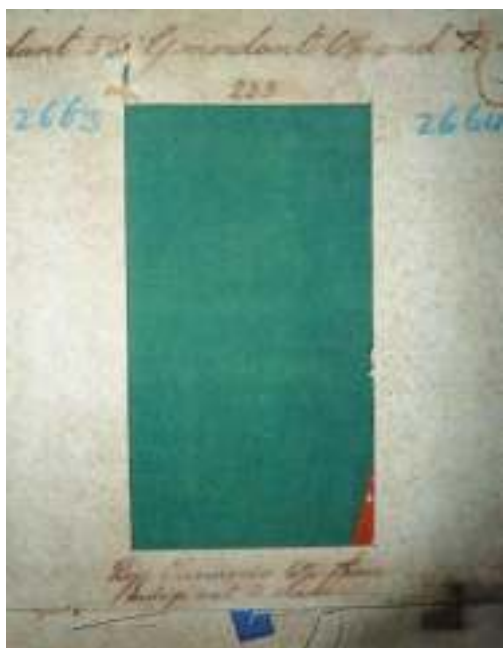
4 A cloth sample dyed with a mixture of turmeric and indigo. Photograph: Jenny Balfour-Paul, courtesy Botanical Survey of India, Kolkata.
