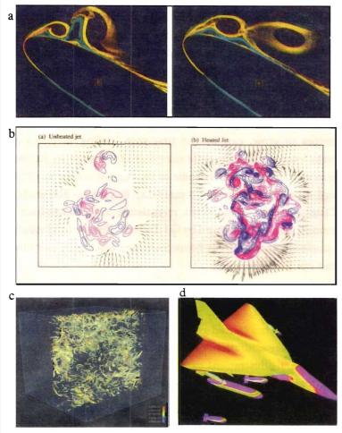
Figure a. Solution of Navier-Stokes equations for an aerofoil at high angle of attach (~29 deg.). Instantaneous contours of vorticy. Reynolds number = 45 000 based on chord.
