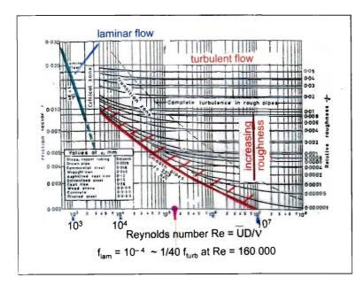
To illustrate the bizarre situation in fluid dynamics, consider the common plumbing problem of estimating the pressure loss suffered by water flowing through a pipe.
