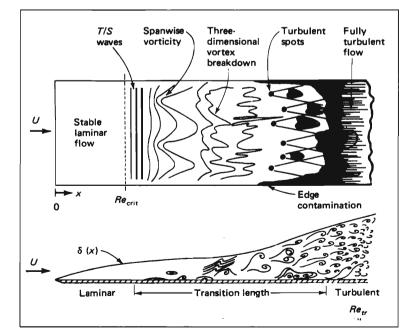
Figure 5. An idealized, schematic picture of how transition from laminar to turbulent flow occurs in the boundary layer on a flat plate, from two-dimensional instability through turbulent spots to fully developed turbulent flow. (Reproduced from Frank M White, Viscous Fluid Flow, McGraw-Hill International Editions, 1991).
