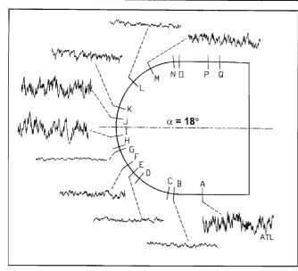
We recently discovered, to our astonishment, that as many as six such transitions – back and forth between laminar and turbulent flow – can occur in a narrow strip around the leading edge of the kind of swept wing that is typical of modern civilian passenger aircraft (such as Boeing and Airbus make). Figure 7 shows how wildly the output from hot-film sensors stuck on the surface of such a wing can vary from one sensor to the next, under conditions typical of take-off or landing.
